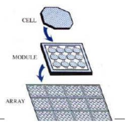
Figure 12.4 Solar Photovoltaic Array
