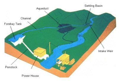
Figure 12.11 Hydro Power Plant
